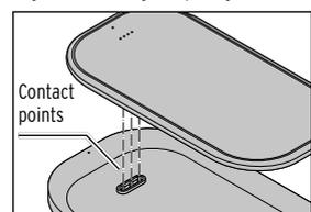
3. Place the power bank on the charging dock as illustrated. The contact points on the power bank and on the charging dock must be facing each other.
